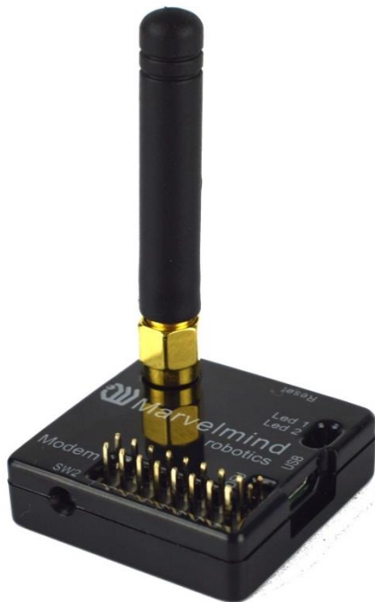
modem v4.9, 915 MHz controller of the system
