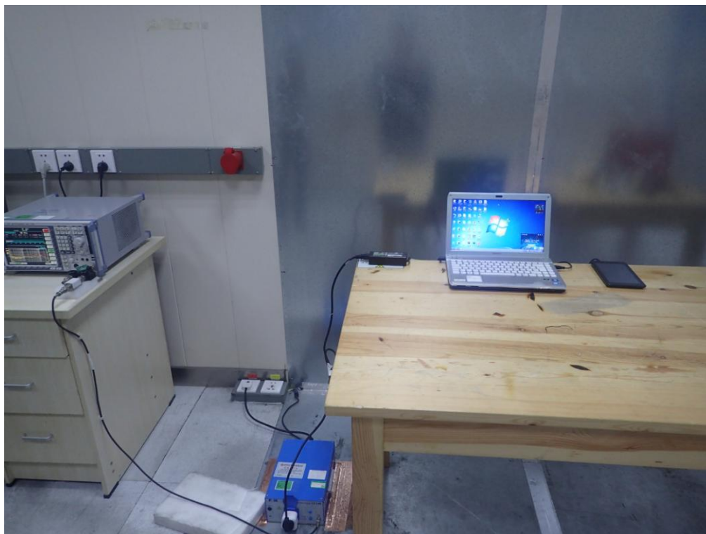
FCC RADIATED EMISSION TEST SETUP
