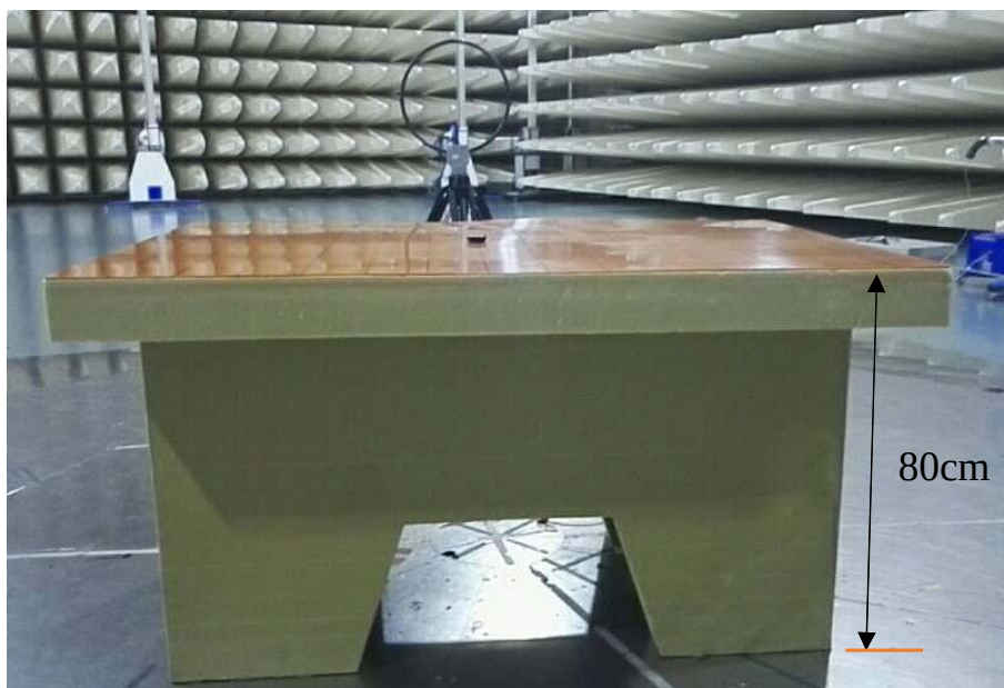
Spurious Radiated Emissions Test setup (below 30MHz)
