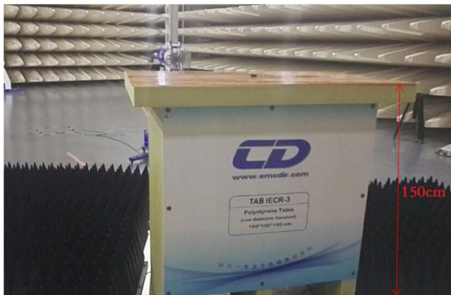
Pic4.Spurious Radiated Emissions Test setup (1GHz~25GHz)
