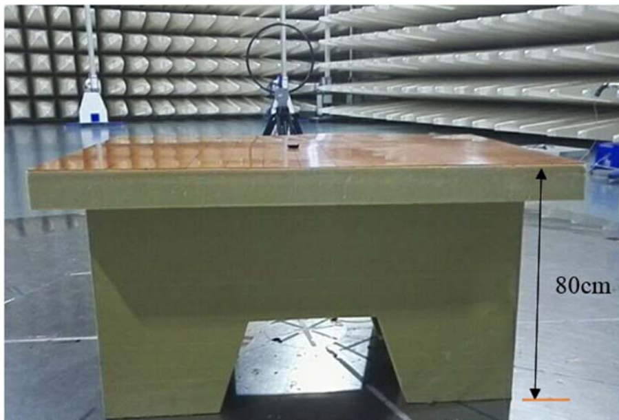
Pic2. Spurious Radiated Emissions Test setup (below 30MHz)
