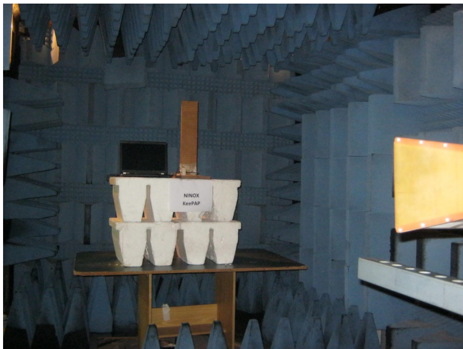
Radiated Emission Test above 1GHz
