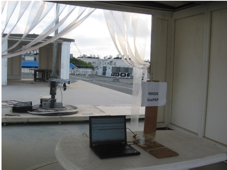
Radiated Emission Test for 200-1000MHz
