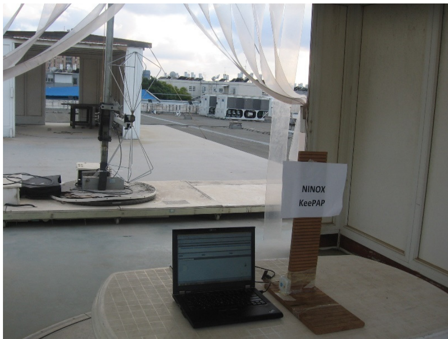
Radiated Emission Test for 30-200MHz
