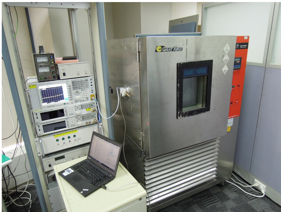
Photograph 5: Set-up for Conducted testing
