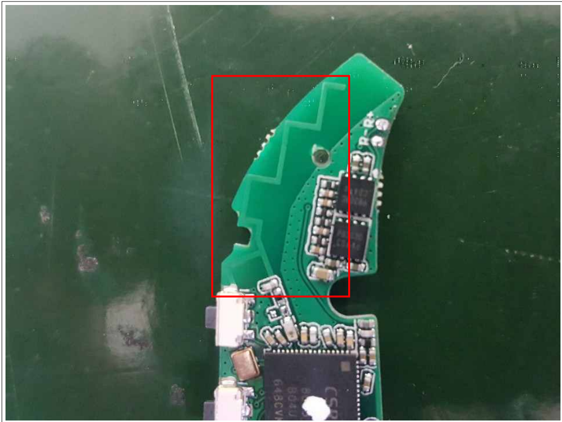
View of Antenna
