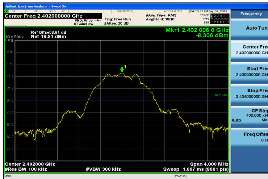
RF Conducted Spurious Emissions_BLE_2402
