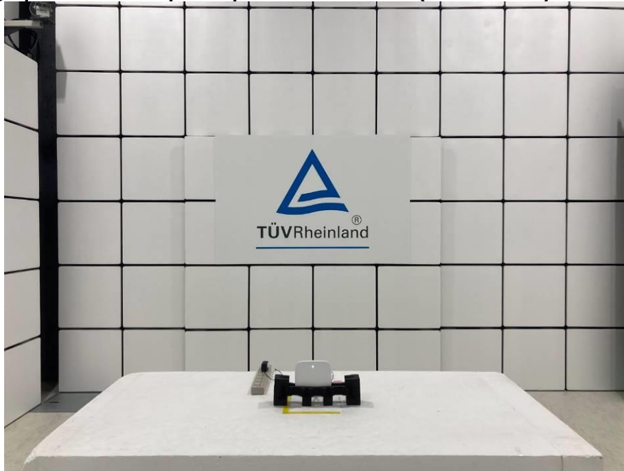
Photograph 1: Test Setup for Spurious Emissions (Front View 1)
