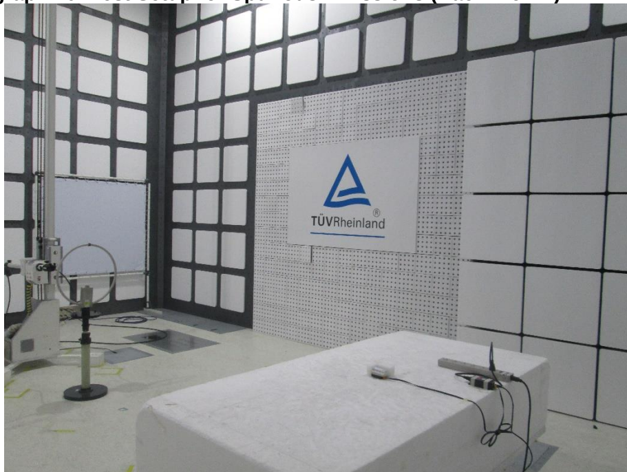
Photograph 10: Test Setup for Spurious Emissions (Back View 1)
