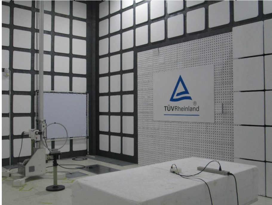
Photograph 3: Test Setup for Spurious Emissions (Back View 1)
