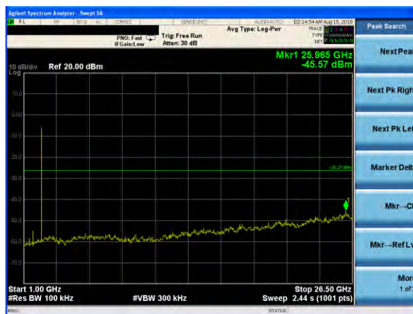
GFSK on channel 00
