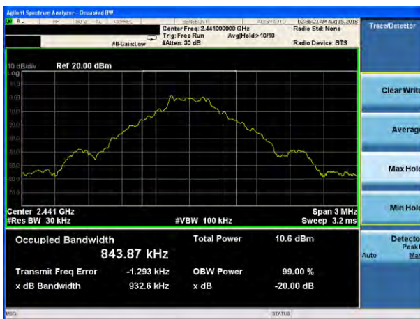
20dB Bandwidth plot on channel 39 (1Mbps)
