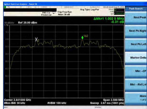
(2Mbps) Channel Separation plot on channel 77-78
