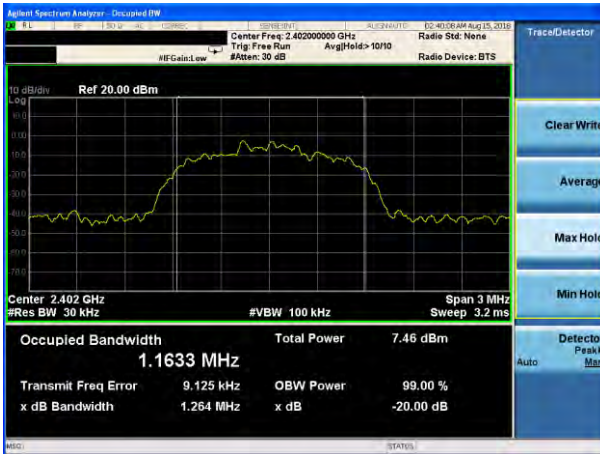
20dB Bandwidth plot on channel 39 (3Mbps)
