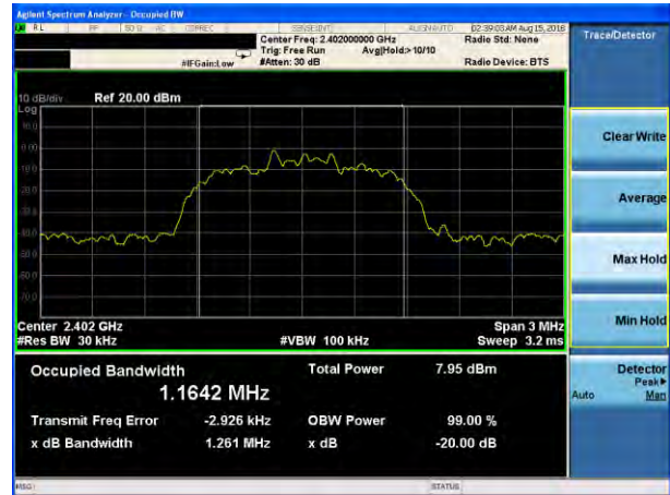
20dB Bandwidth plot on channel 39 (2Mbps)
