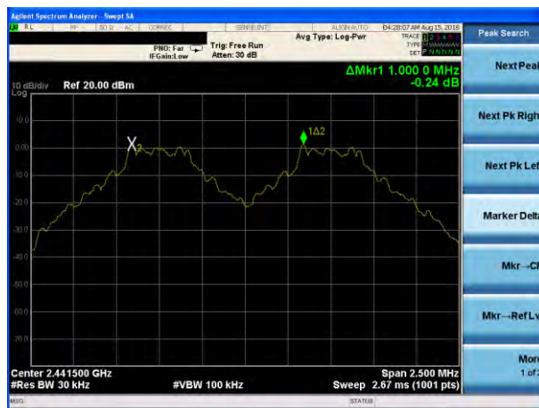
(1Mbps) Channel Separation plot on channel 77-78
