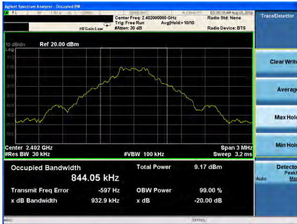
20dB Bandwidth plot on channel 39 (1Mbps)
