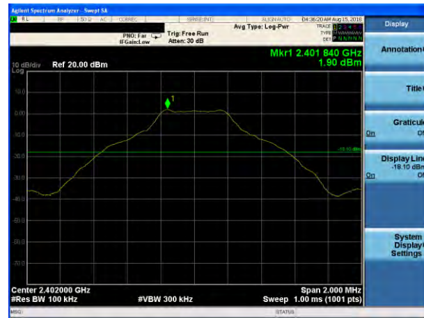
GFSK on channel 00
