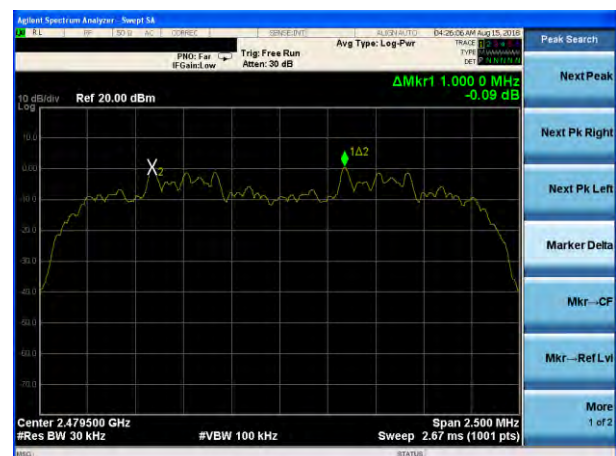
(2Mbps) Channel Separation plot on channel 77-78
