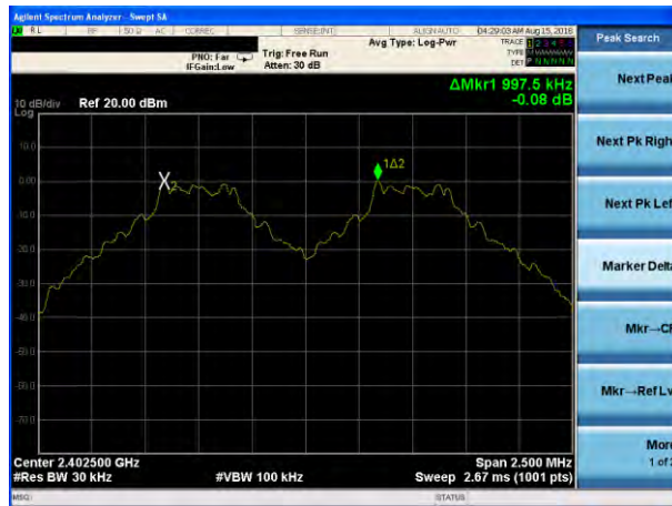
(1Mbps) Channel Separation plot on channel 39-40
