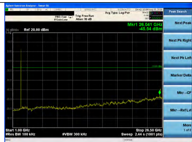
GFSK on channel 39
