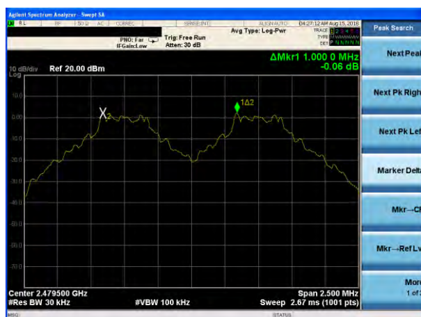
(1Mbps) Channel Separation plot on channel 77-78
