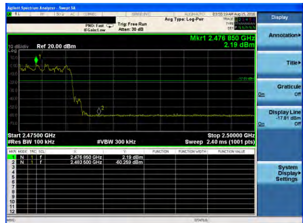
\pi/4 -DQPSK: Band Edge-High Channel (Hopping Mode)
