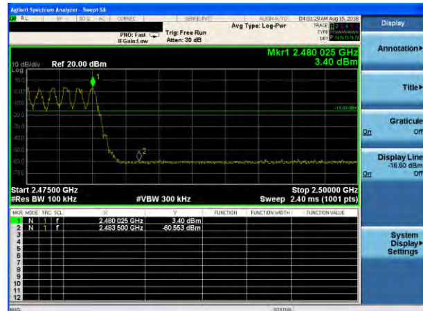
GFSK: Band Edge-High Channel (Hopping Mode)
