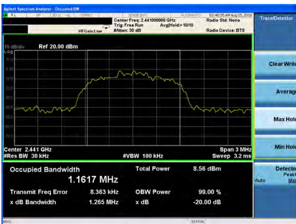
20dB Bandwidth plot on channel 39 (3Mbps)
