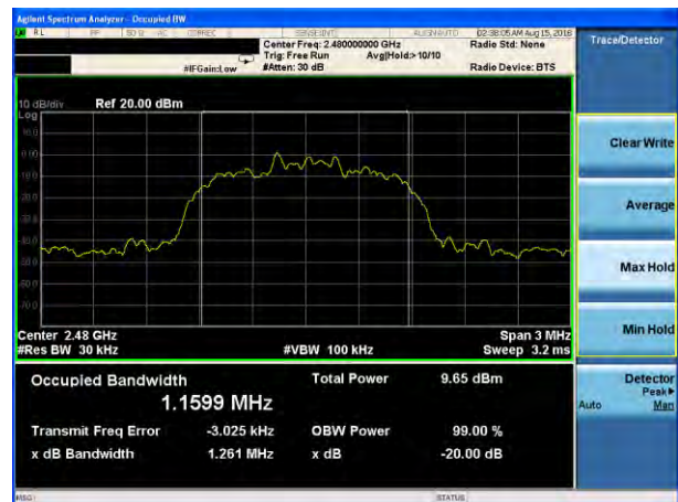
20dB Bandwidth plot on channel 78 (2Mbps)
