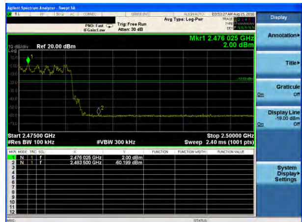
8-DPSK: Band Edge-High Channel (Hopping Mode)
