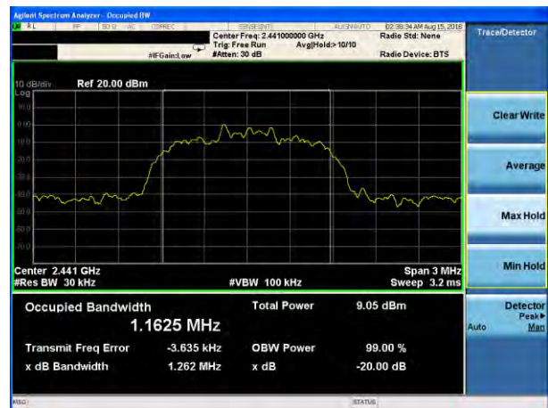
20dB Bandwidth plot on channel 39 (2Mbps)
