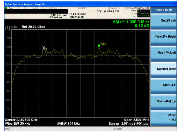
(2Mbps) Channel Separation plot on channel 39-40
