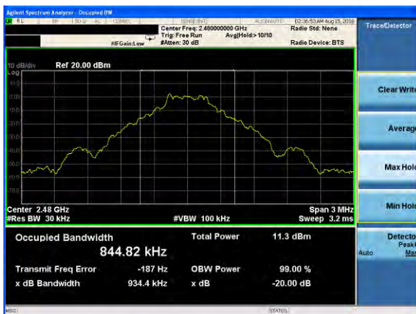
20dB Bandwidth plot on channel 78 (1Mbps)
