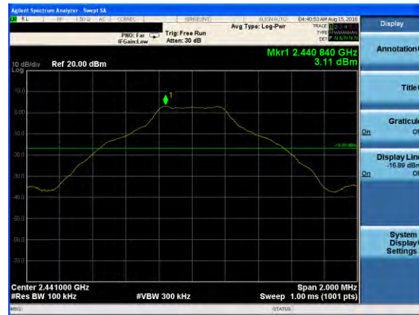
GFSK on channel 39
