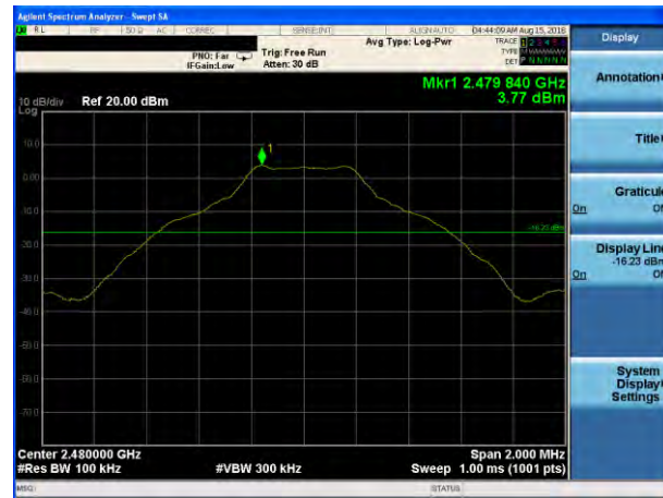
GFSK on channel 78
