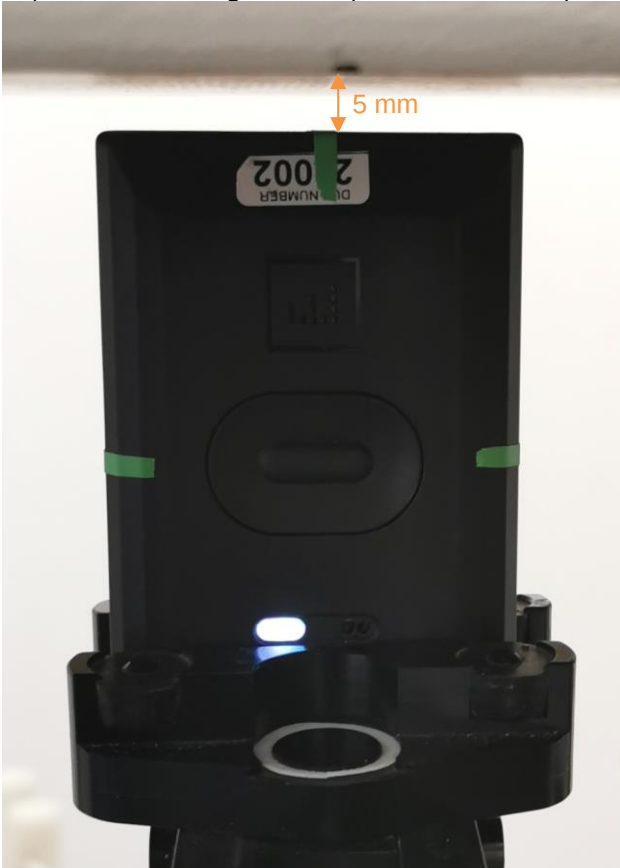
Bottom of the device against the phantom, 5mm separation distance
