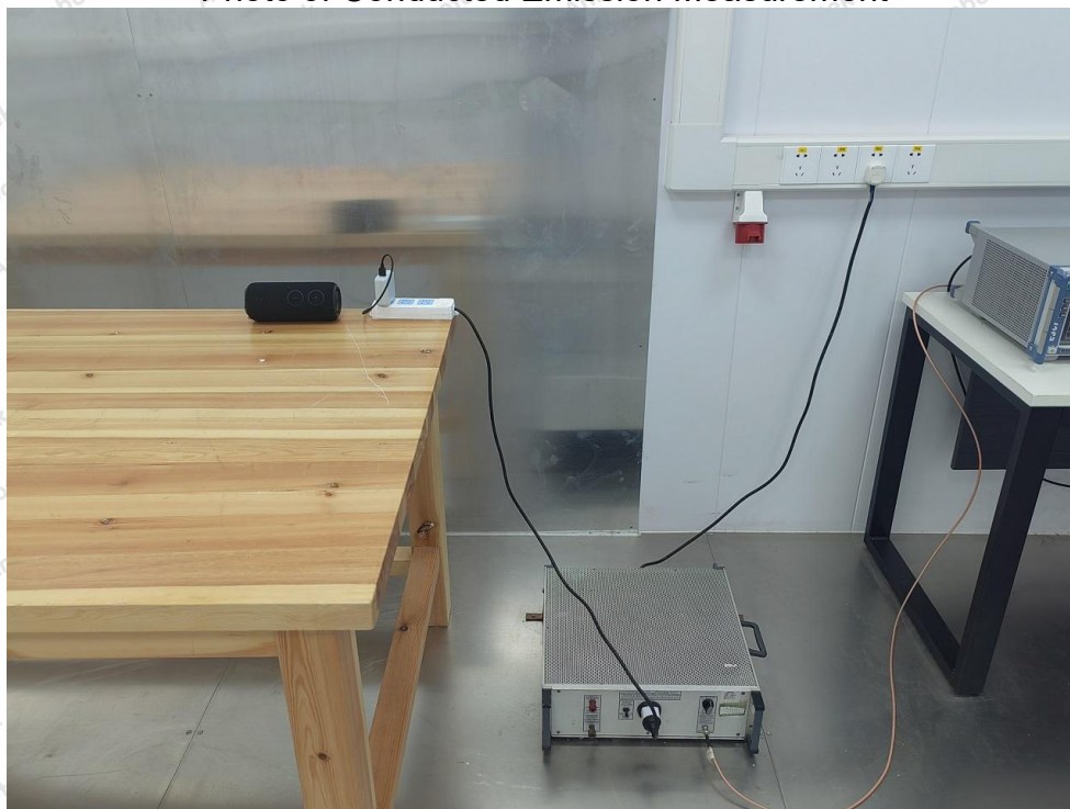
Photo of Conducted Emission Measurement
