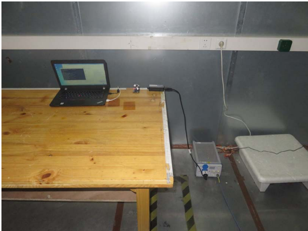
Picture 3 Conducted Emission Test Setup
