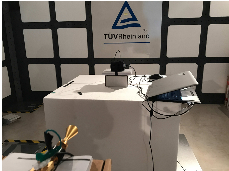
Photograph 4: Set-up for Spurious Emissions (Above 40GHz)
