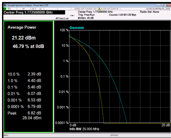
Band66 QPSK BW=15MHz Channel=132597 RB Size=75 Position=#0
