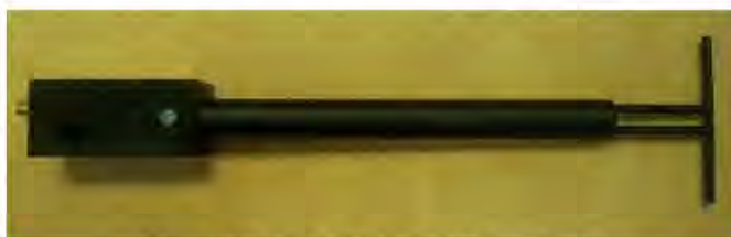
Figure 1 – MVG COMOSAR Validation Dipole
