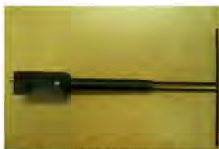
Figure 1 – MVG COMOSAR Validation Dipole
