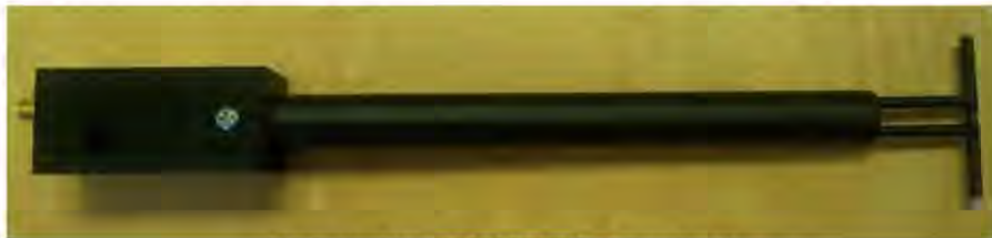
Figure 1 – MVG COMOSAR Validation Dipole
