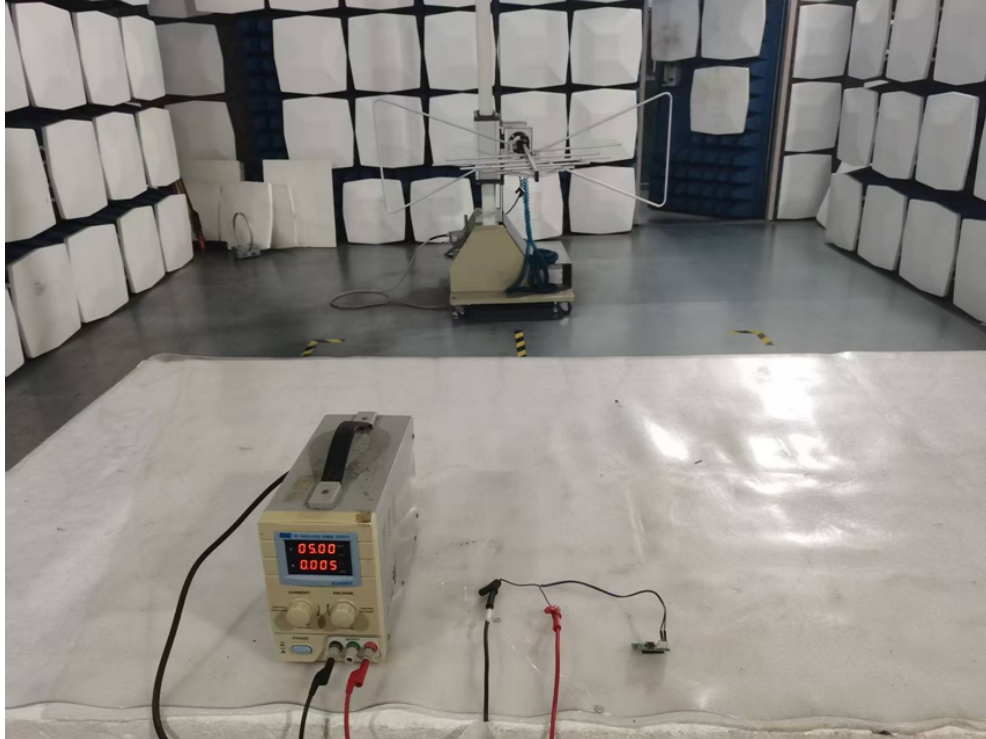
Radiated Emission Test Setup:
