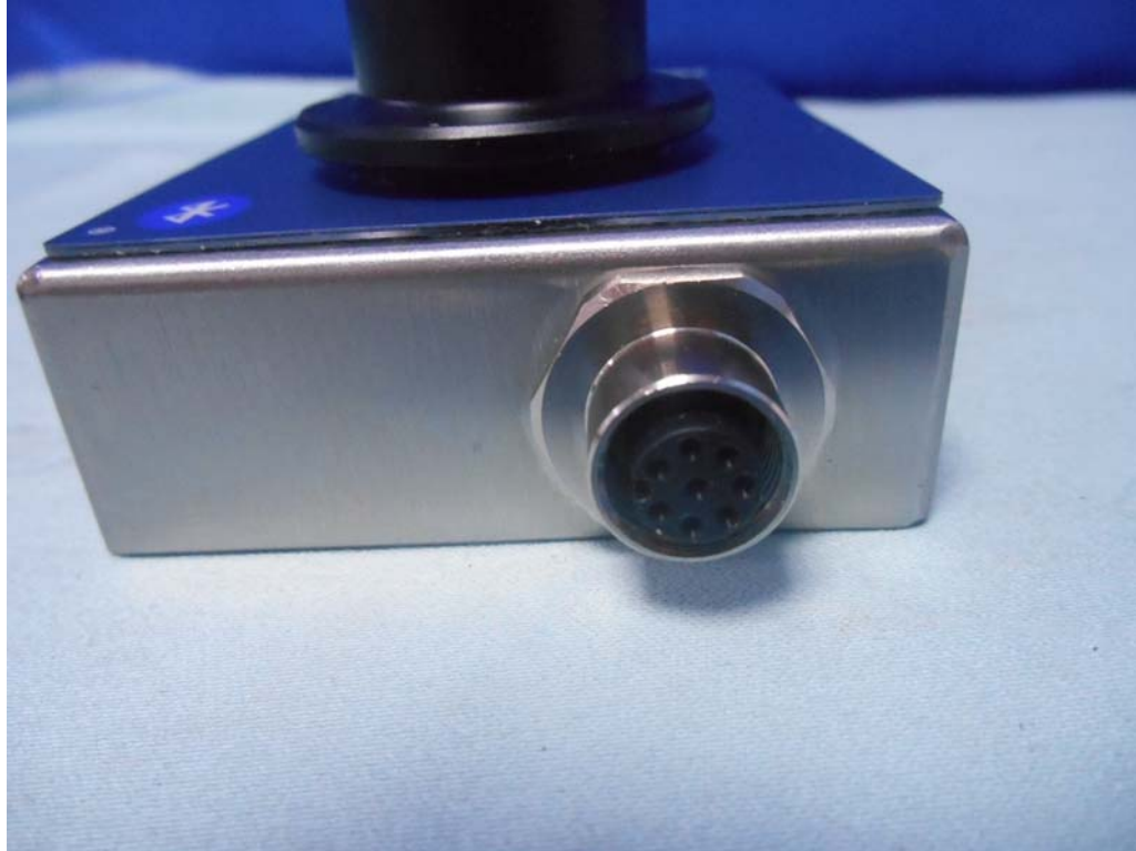
FIGURE 3 BLUETOOTH MODULE ACW520 (M/N: ACW520-BT) GENERAL APPEARANCE (INTERFACE PORT)
