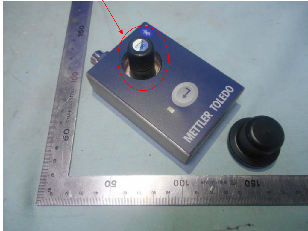
FIGURE 4 BLUETOOTH MODULE ACW520 (M/N: ACW520-BT) ANTENNA LOCATION
