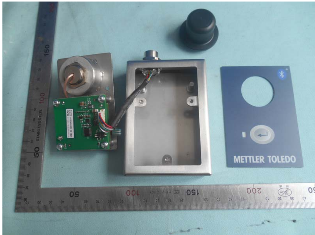
FIGURE 5 BLUETOOTH MODULE ACW520 (M/N: ACW520-BT) COVER REMOVED
