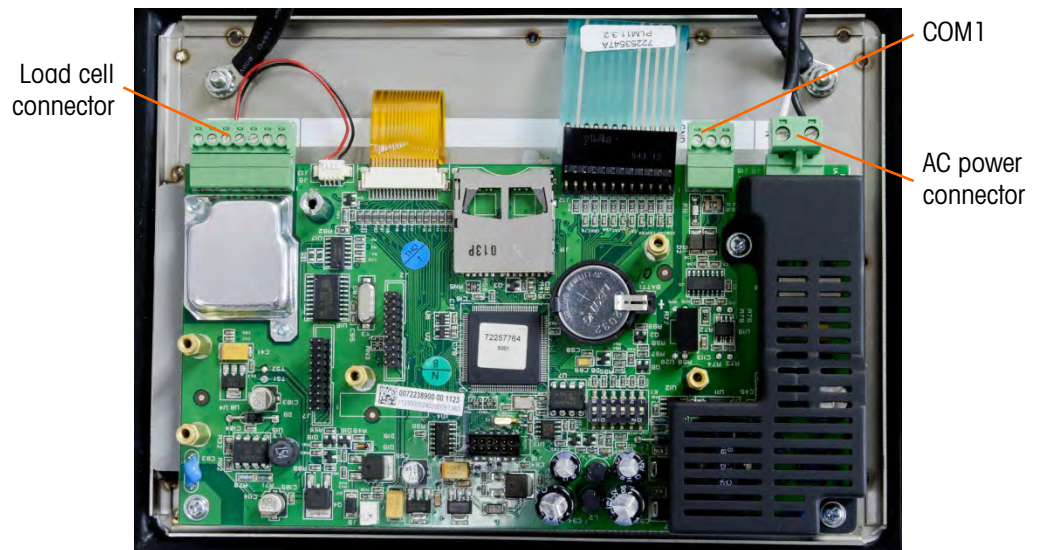
Figure 2-19: IND246 Main Board Connections, AC Model
