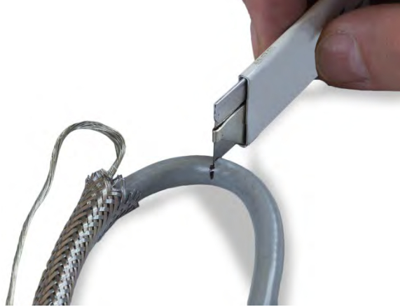
Figure 2-33: Cutting Around Cable Jacket
