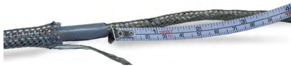
Figure 2-36: Marking the Inner Braided Shield
