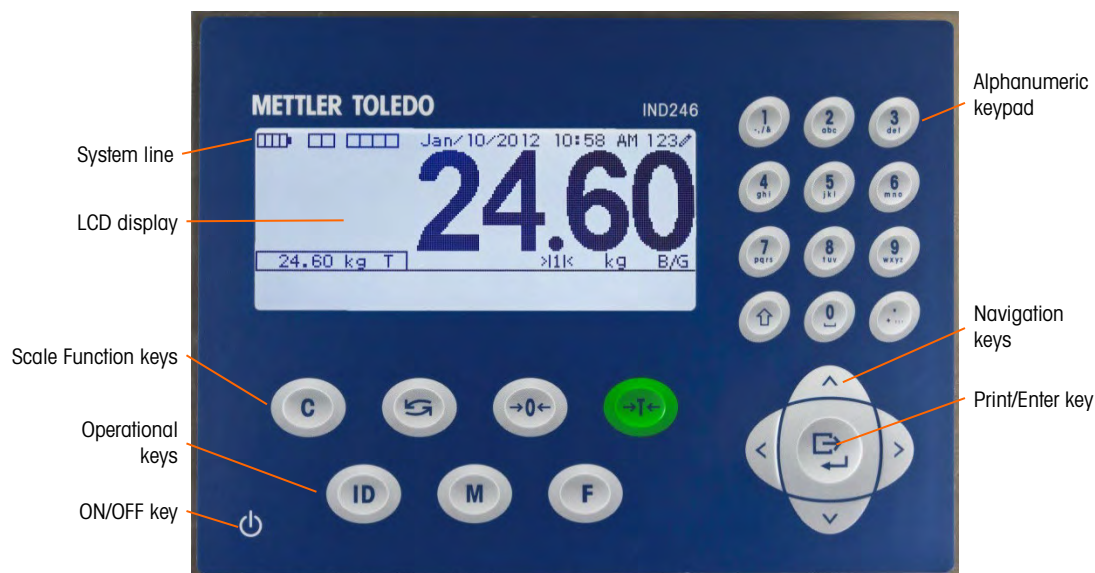
Figure 1-5: IND246 Front Panel Layout
