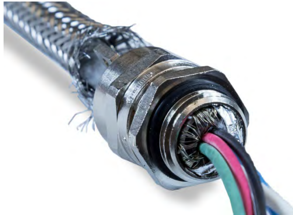
Figure 2-45: Inner Armor and Foil Pressed into Body of Cable Gland
