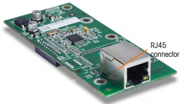
Figure 2-61: Ethernet Connection Option Board
