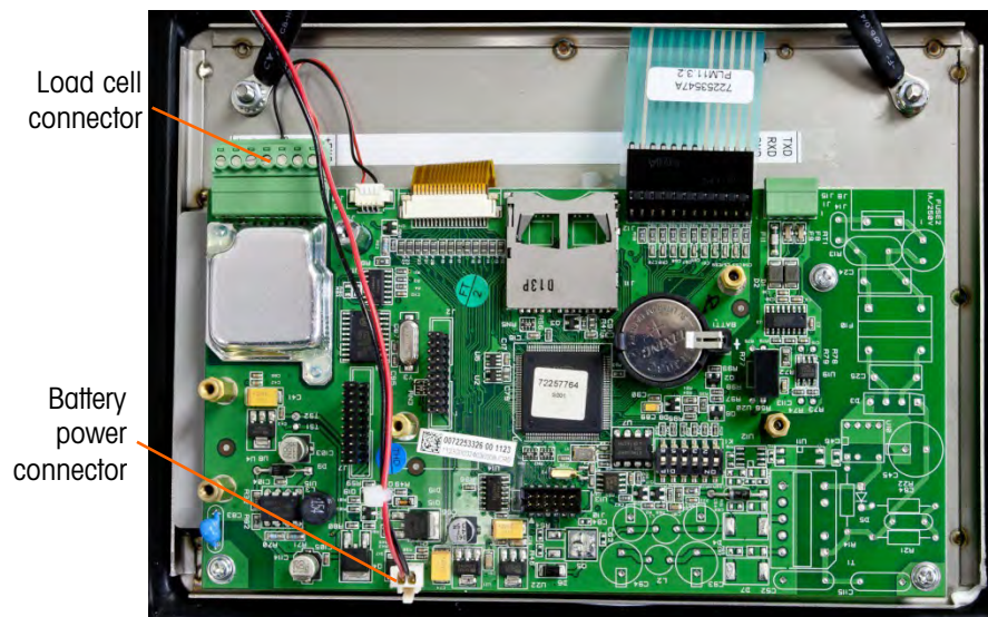
Figure 2-20: IND246 Main Board Connections, Battery-Powered Model
