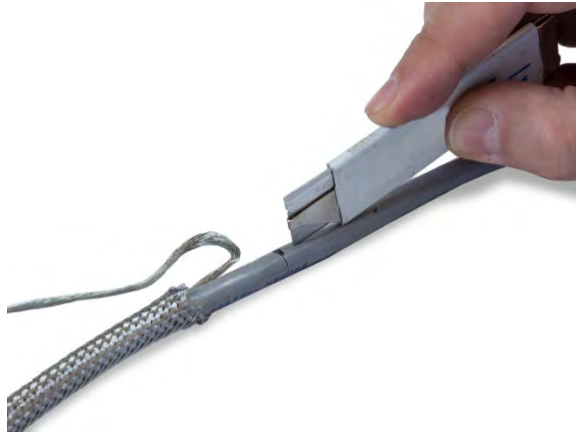
Figure 2-34: Cutting Along the Cable Jacket
