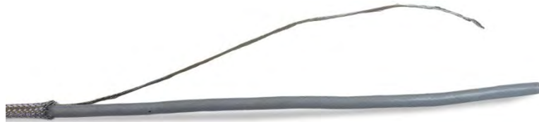
Figure 2-31: Exterior Braided Armor Trimmed Back
