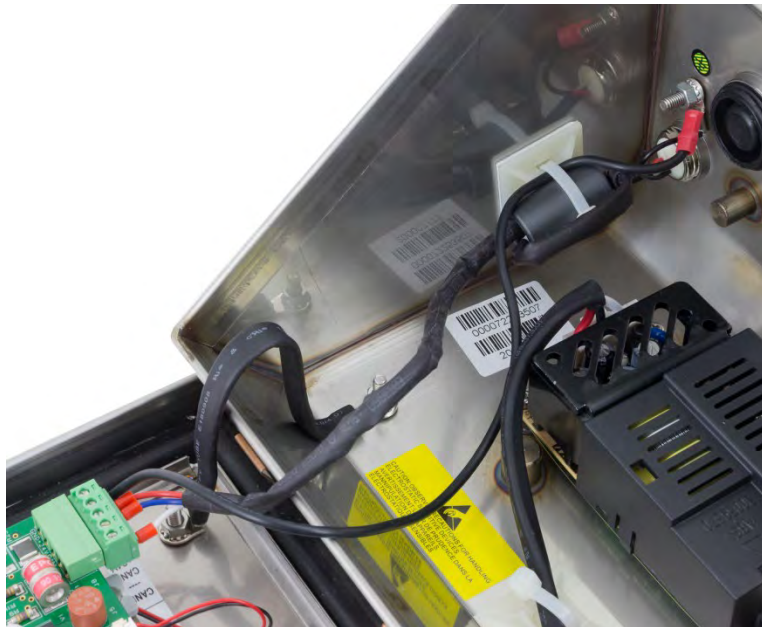
Figure 2-56: PowerDeck Connector Installed in the IND246 POWERCELL
