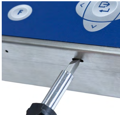
Figure 2-1: Opening the Harsh Enclosure
