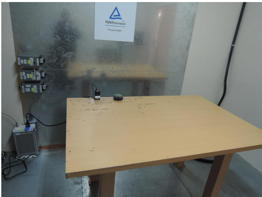
Photograph 5: Set-up for for Mains Conducted testing Front
