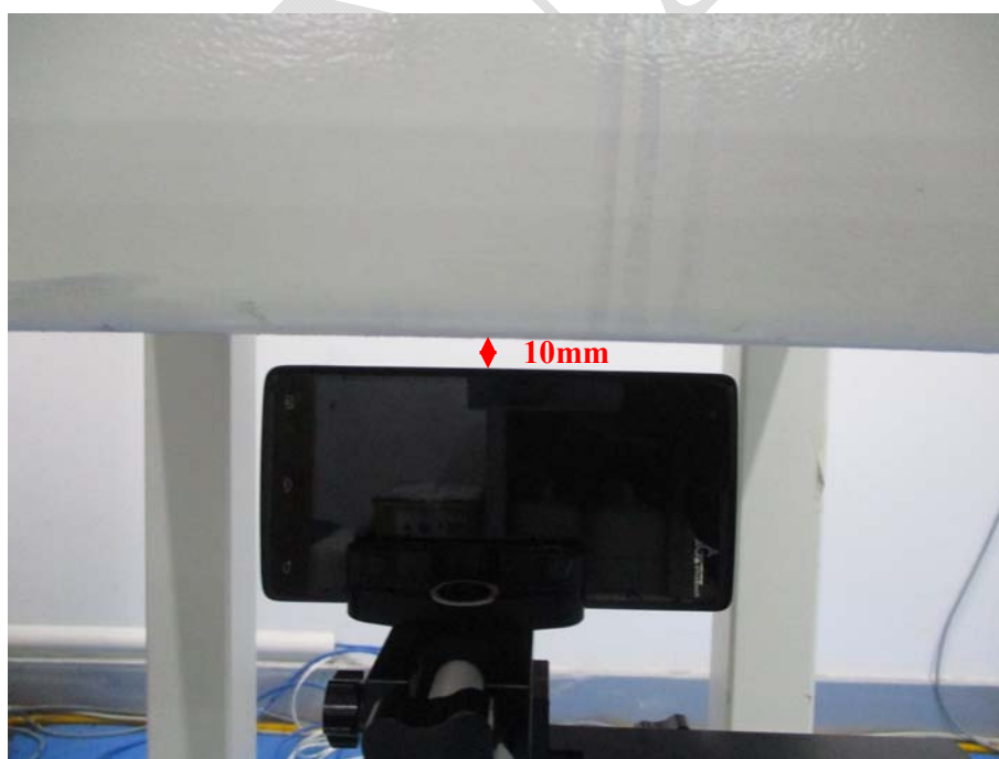
Body Left Setup Photo(10mm)
