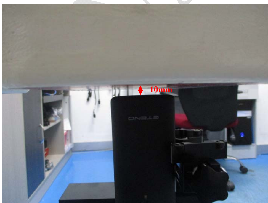
Body Bottom Setup Photo(10mm)
