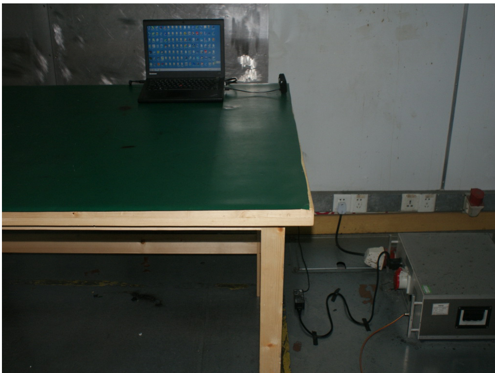
Photograph 6: Set-up for Conducted Emissions
