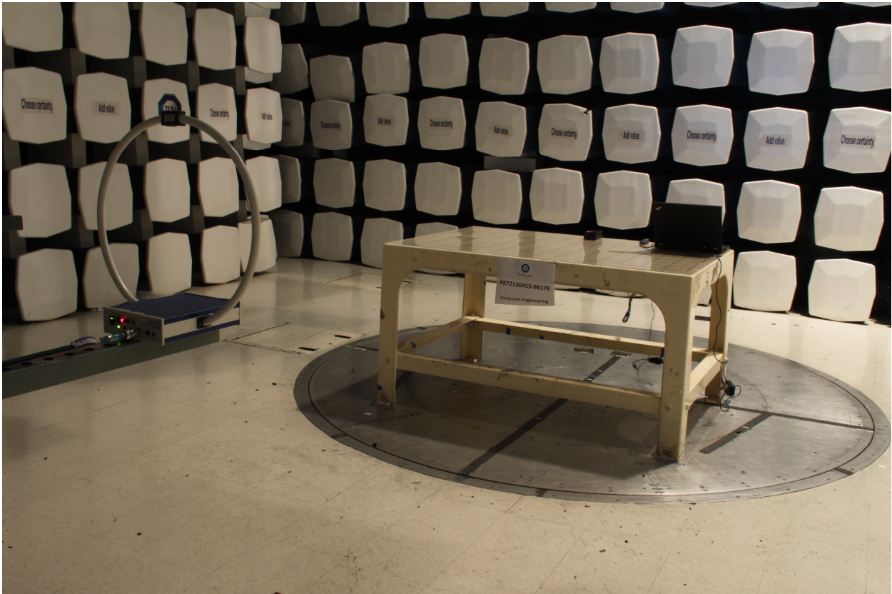
Below 30 MHz Test Setup
