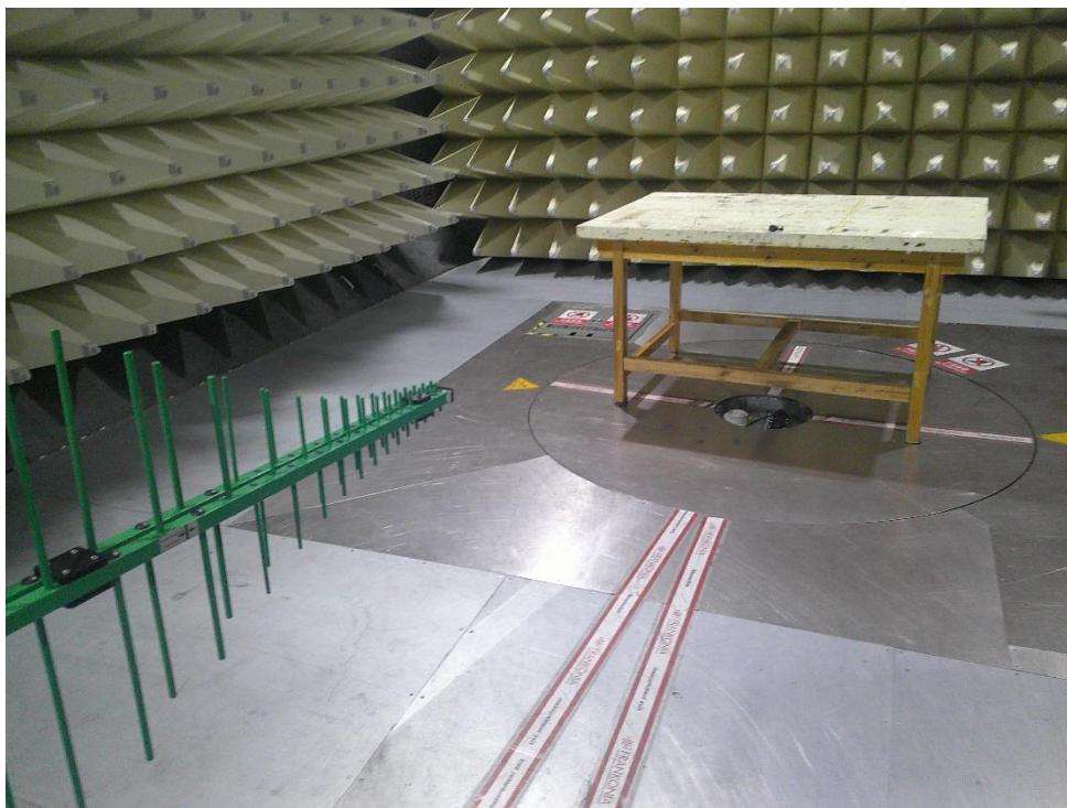
Photograph 1: Set-up photo for Radiated Emission, 30MHz - 1GHz
