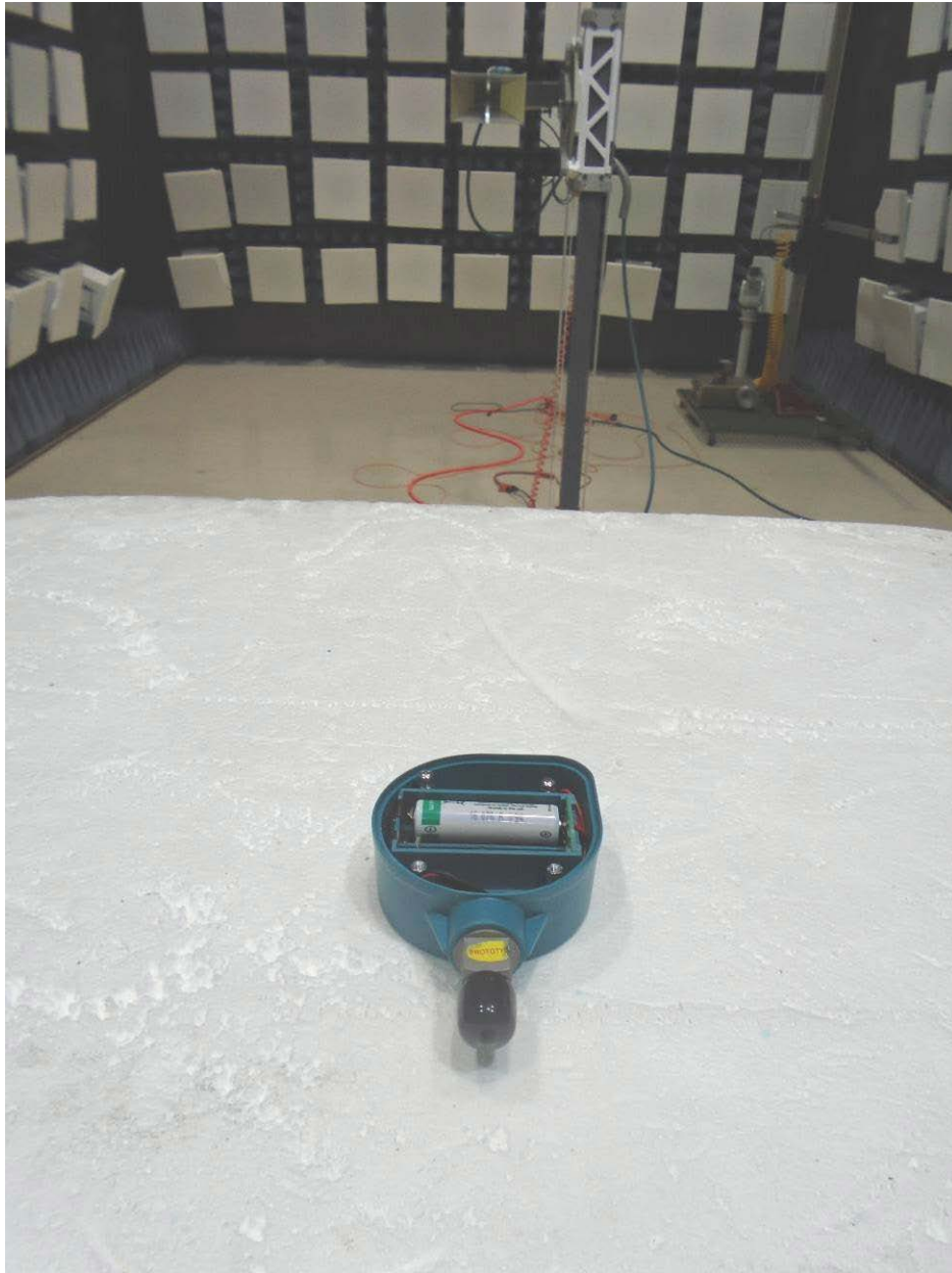
Figure 6: Radiated Emissions – Orientation C Investigation for highest emissions
