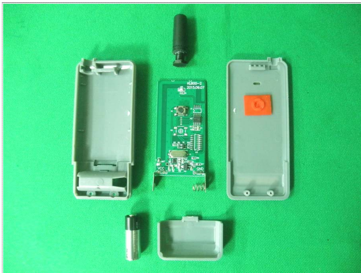
Inner View of TX
