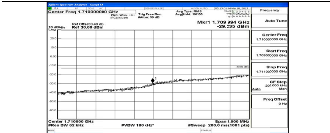
(Channel Bandwidth: 5 MHz)_LCH_16QAM_12RB#13
