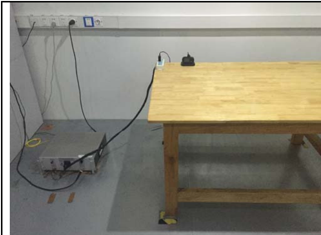
Conducted Emissions Test Setup – Front View
