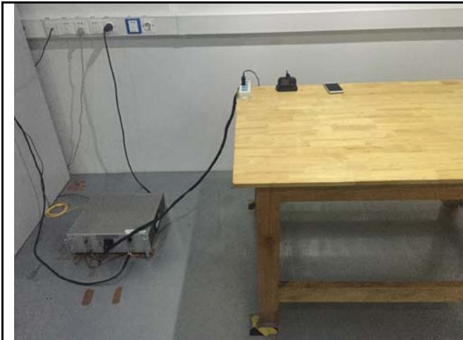
Conducted Emissions Test Setup Front View
