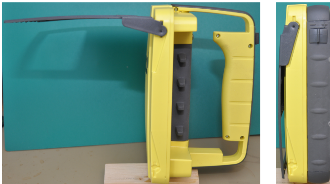
Figure 5: Recco detector right view, antenna and handle opened(left)/closed(right)
