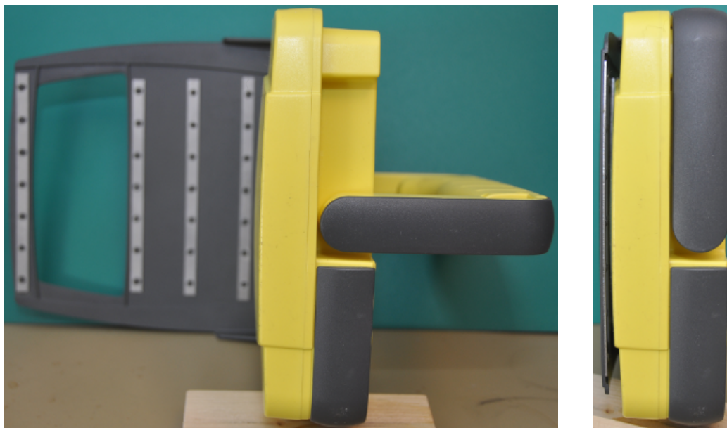
Figure 7: Recco detector bottom view, antenna and handle opened(left)/closed(right)
