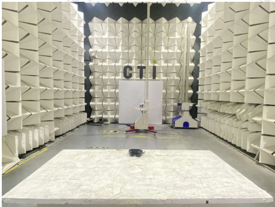
Radiated spurious emission Test Setup-1(Below 1GHz)
