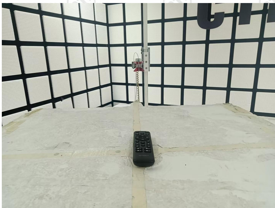
Radiated spurious emission Test Setup-3(Above 1GHz)
