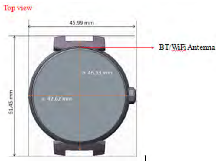
Fig.6 Antenna location (Front view)
