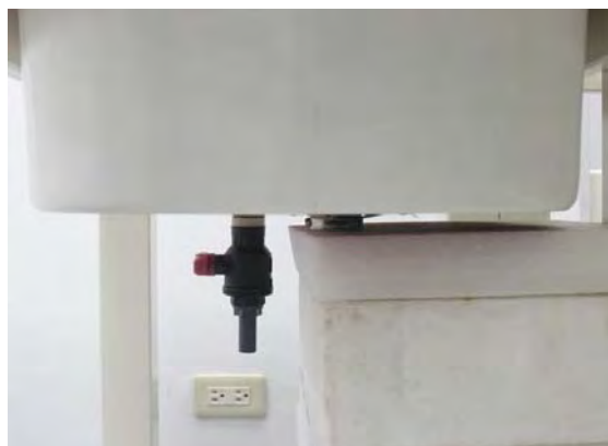
Fig.4 EUT (QA08) Back side to flat phantom
