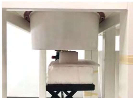
Fig.5 EUT (QA05 change the watchband) Back side to flat phantom
