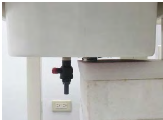
Fig.3 EUT (QA05) Back side to flat phantom
