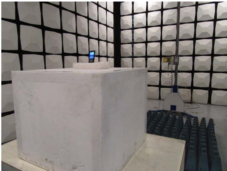
Radiated Emission View (Above 1GHz)
