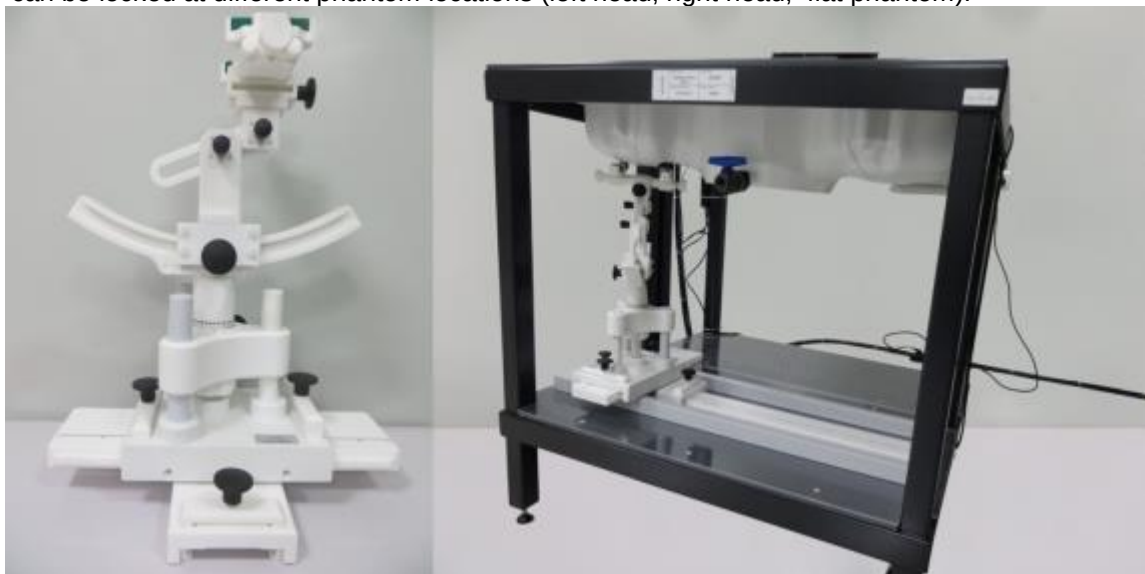
Device holder supplied by SATIMO
