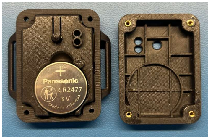
Figure 4-1: Removing Battery Lid from eBeat
