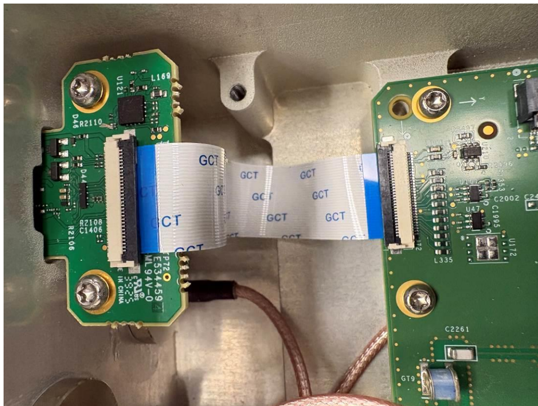
Close-up view of Ethernet / Power interface
