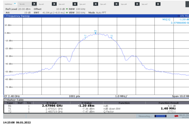
Figure 8.4-3: 6 dB bandwidth on High ch.
