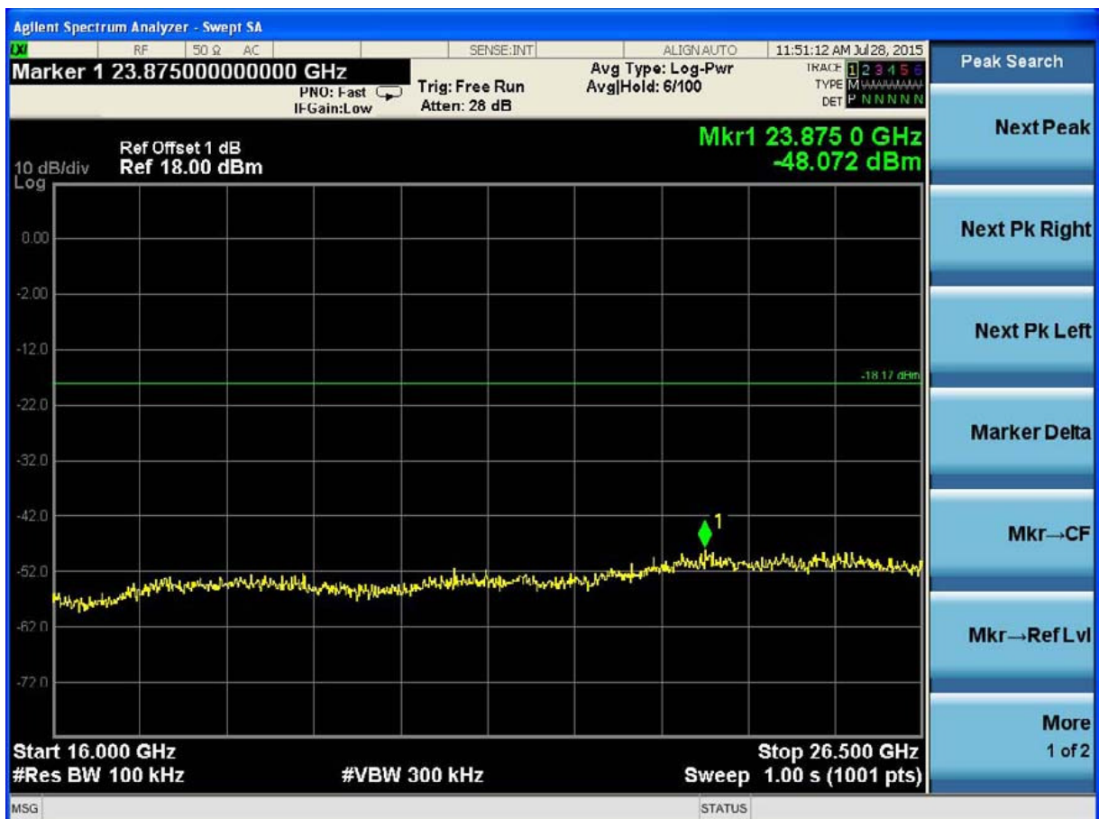
(Plot 4.7.1 C6: Channel 78: 2480MHz @ GFSK)
