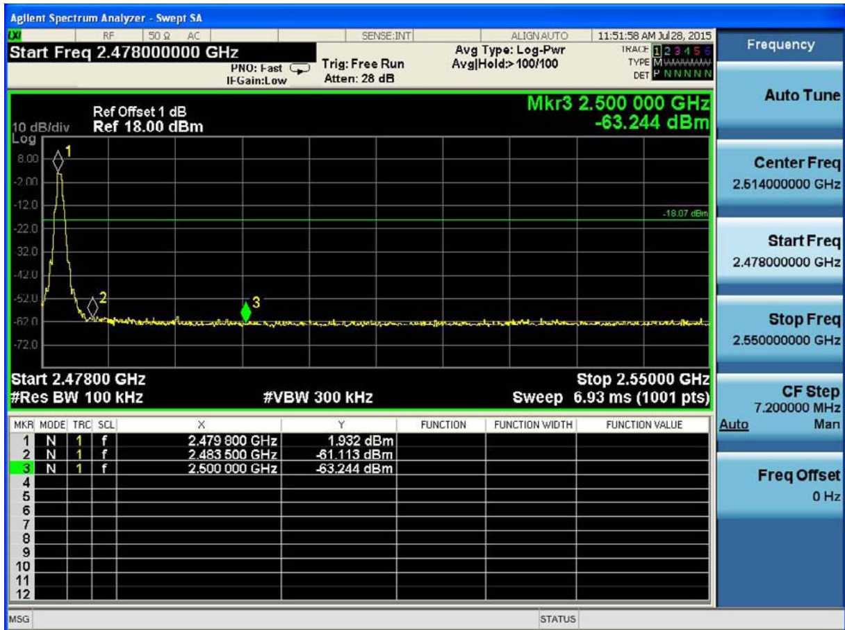
(Plot 4.6.2.1 C: Channel 78: 2480MHz @ GFSK)
