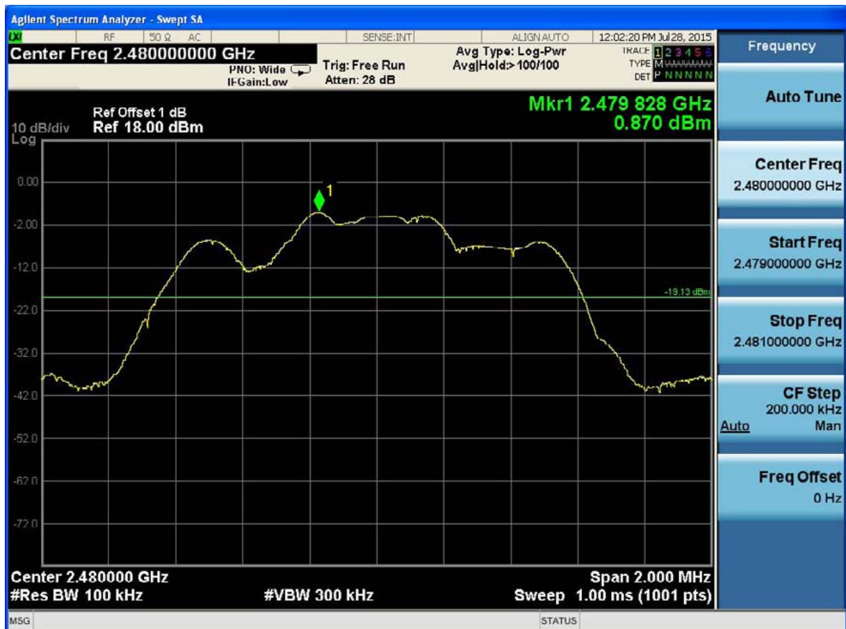
(Plot 4.7.2 C1: Channel 78: 2480MHz @8DPSK)
