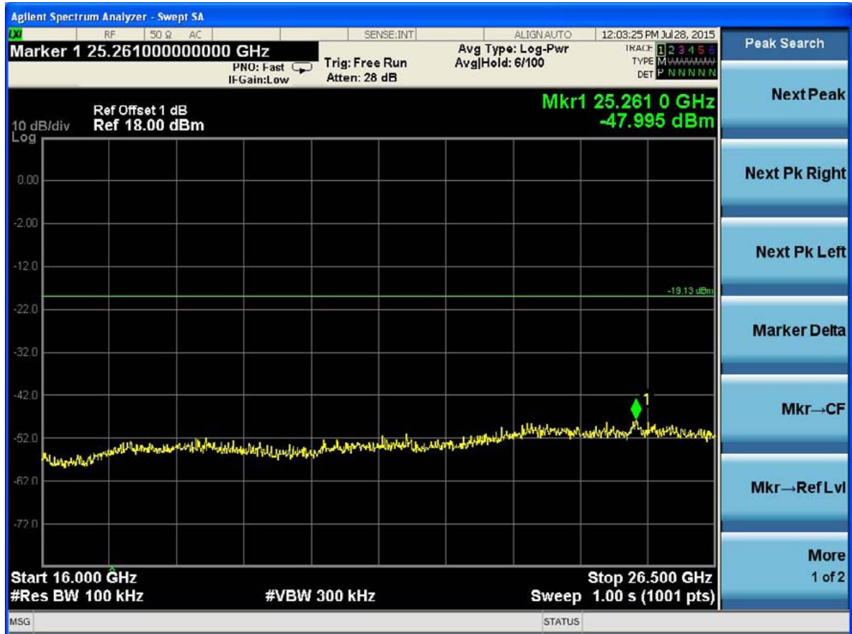
(Plot 4.7.2 C6: Channel 78: 2480MHz @8DPSK)
