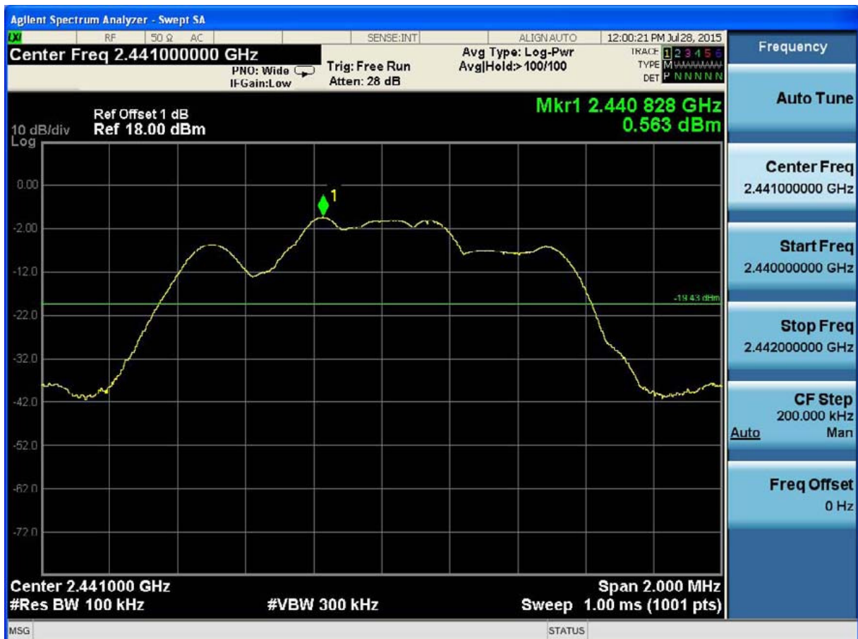
(Plot 4.7.2 B1: Channel 39: 2441MHz @8DPSK)
