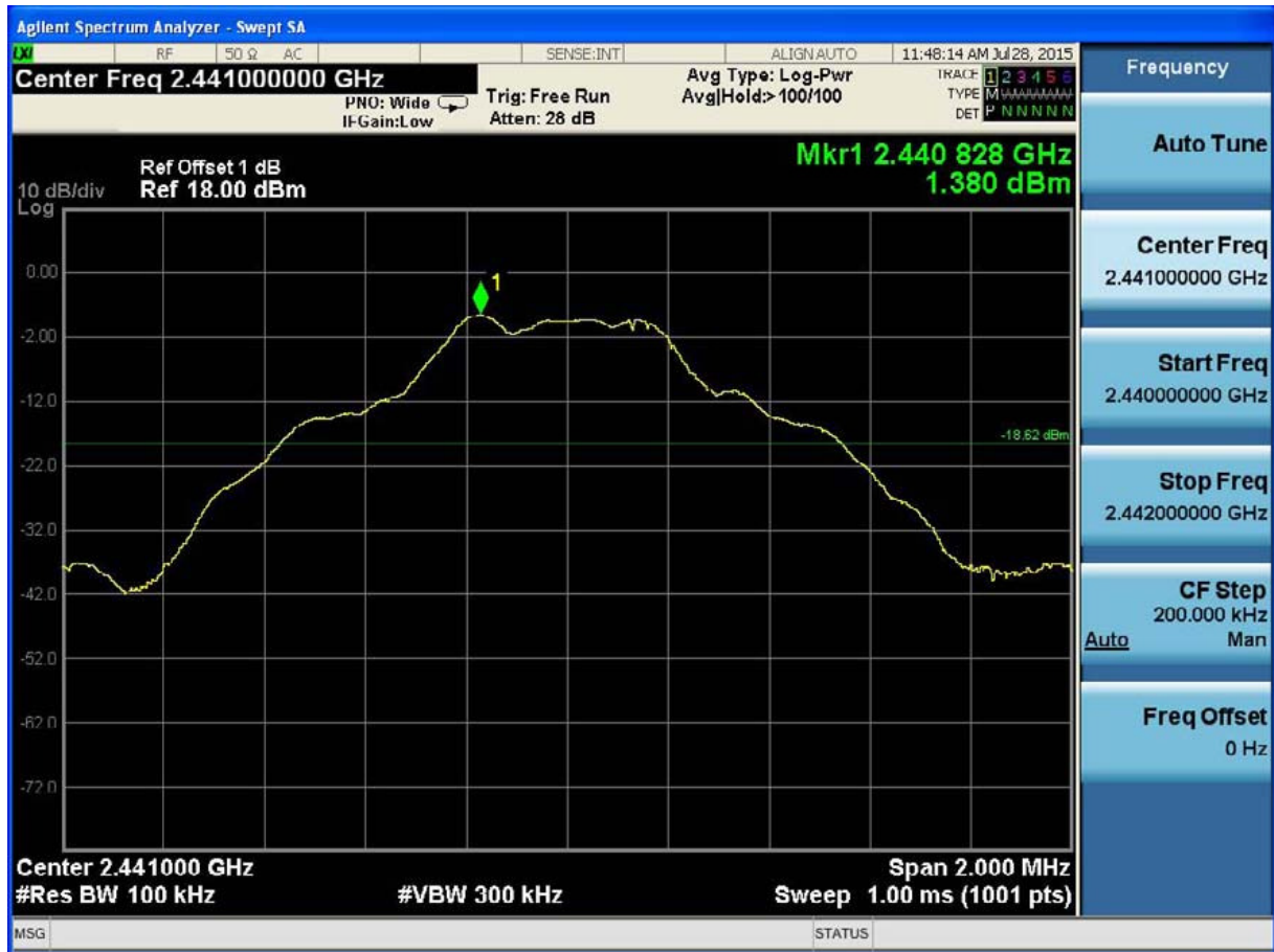
(Plot 4.7.1 B1: Channel 39: 2441MHz @ GFSK)
