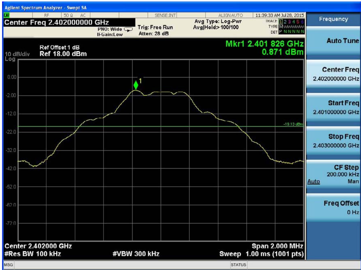
(Plot 4.7.1 A1: Channel 00: 2402MHz @ GFSK)
