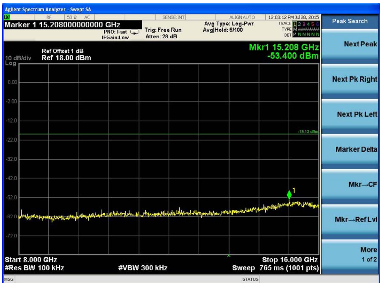
(Plot 4.7.2 C5: Channel 78: 2480MHz @8DPSK)
