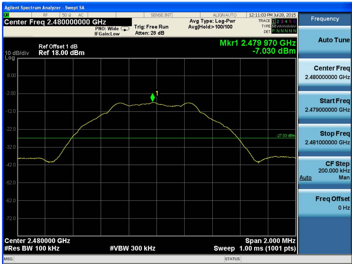
(Plot 4.7.1 C1: Channel 39: 2480MHz @ GFSK)
