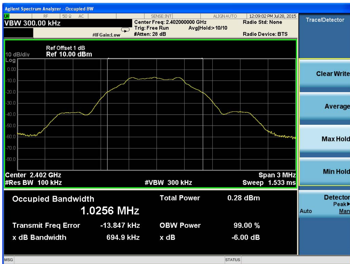
(Plot 4.5.1 A: Channel 00: 2402MHz @ GFSK)
