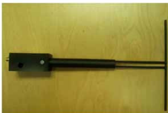
Figure 1 – MVG COMOSAR Validation Dipole
