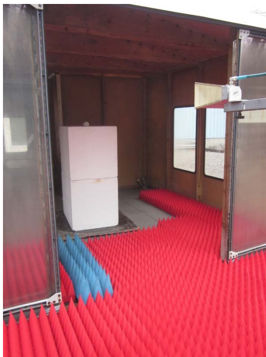
Vertical Antenna Polarization, 1 GHz to 12 GHz, Double Ridge Guide
