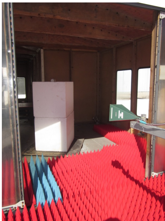
Horizontal Antenna Polarization, 12 GHz to 18 GHz, High Gain Horn Antenna
