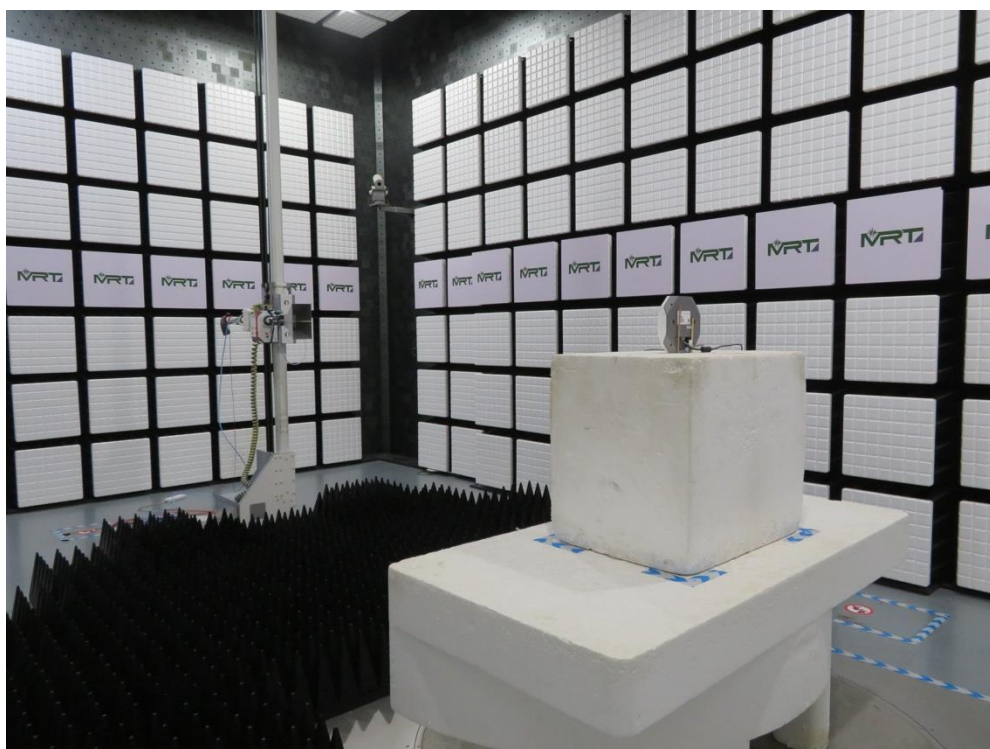
Description: Radiated Spurious Emission Test Setup for Above 1GHz
