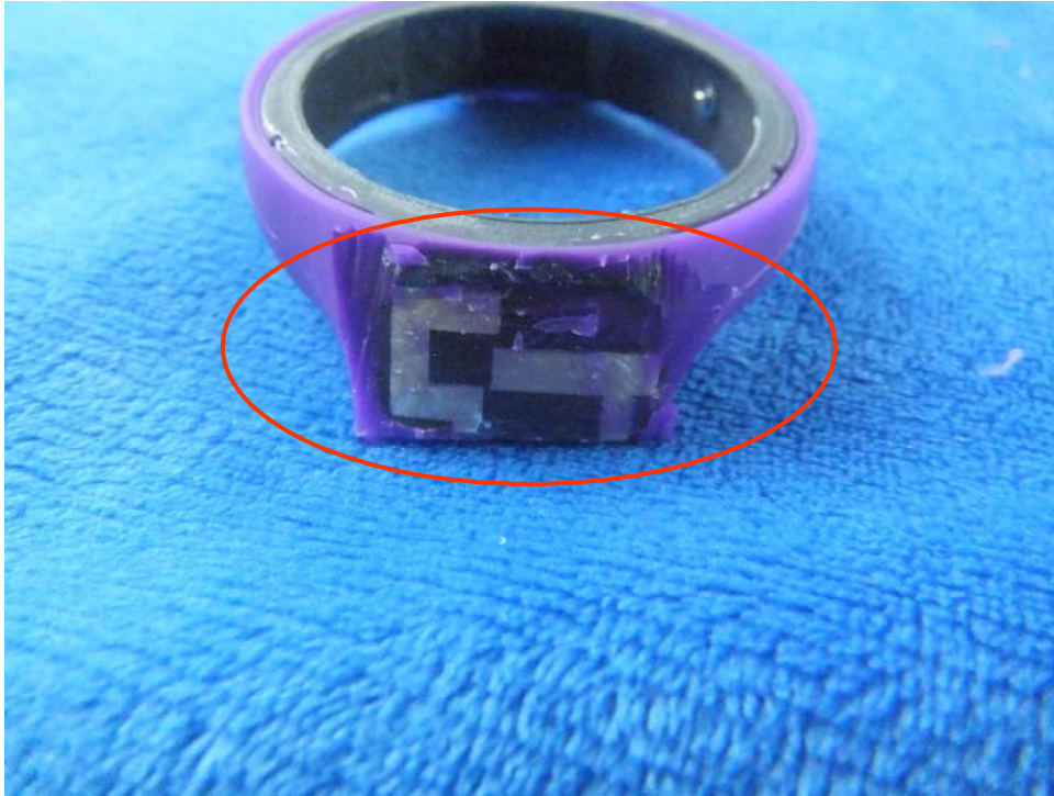
GSM/PCS/UMTS-FDD Antenna View
