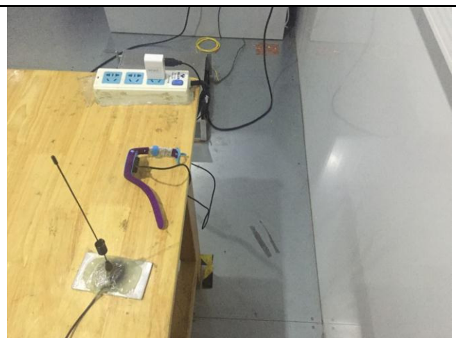
Conducted Emissions Test Setup Side View
